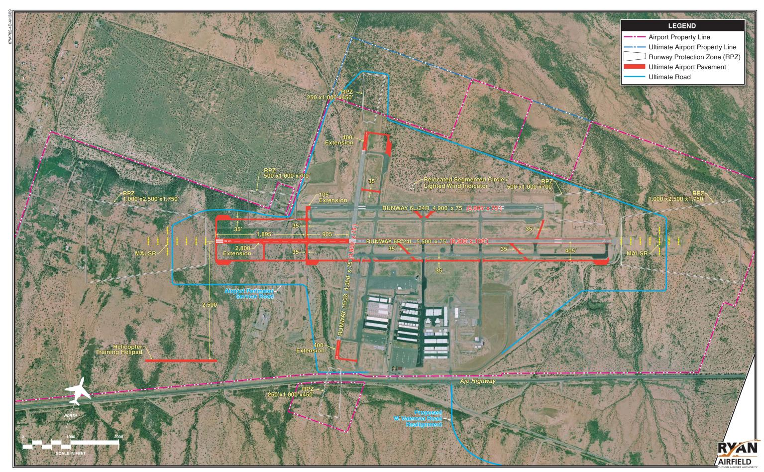
timate Runway 6R end. This could help reduce taxiway congestion on Taxiway B by providing an alternate route to the Runway 6R threshold. A disadvantage of this would be that Taxiway A would lay within the Runway 6L RPZ.
